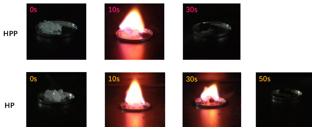
Figure S3 Flame retardancy performance diagrams of HPP and HP.
