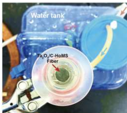
Figure S4. Continuous flow cell for photothermal enhanced uranium extraction.
